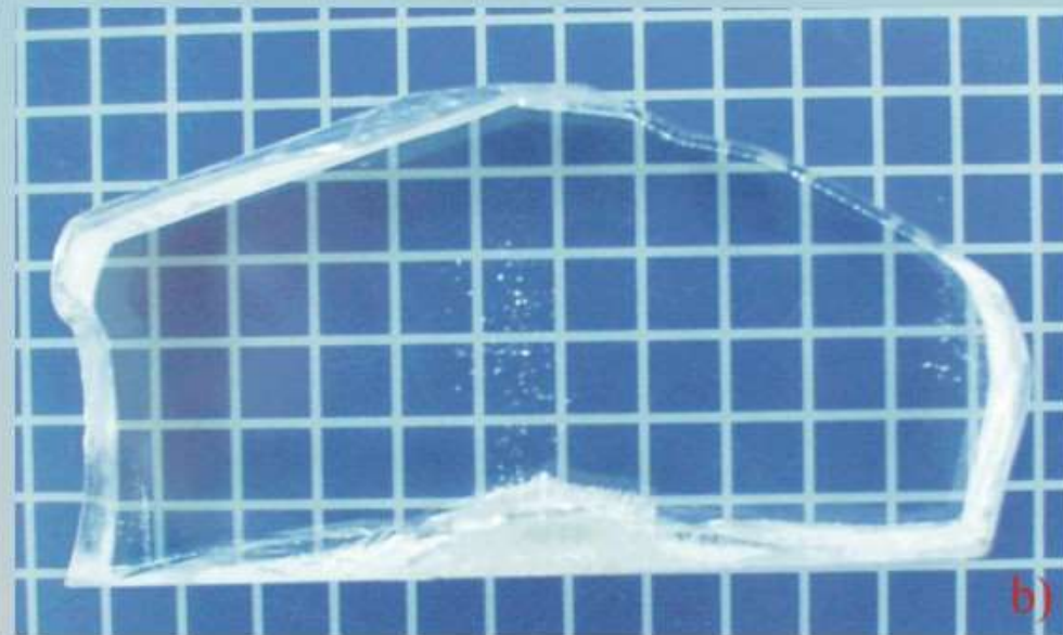
Fig. 3. Side view (a) and axial section of BBO crystal 16 mm in thickness (b) grown under heat field of qL 3 symmetry. Cell size is 5x5 mm 2 .
