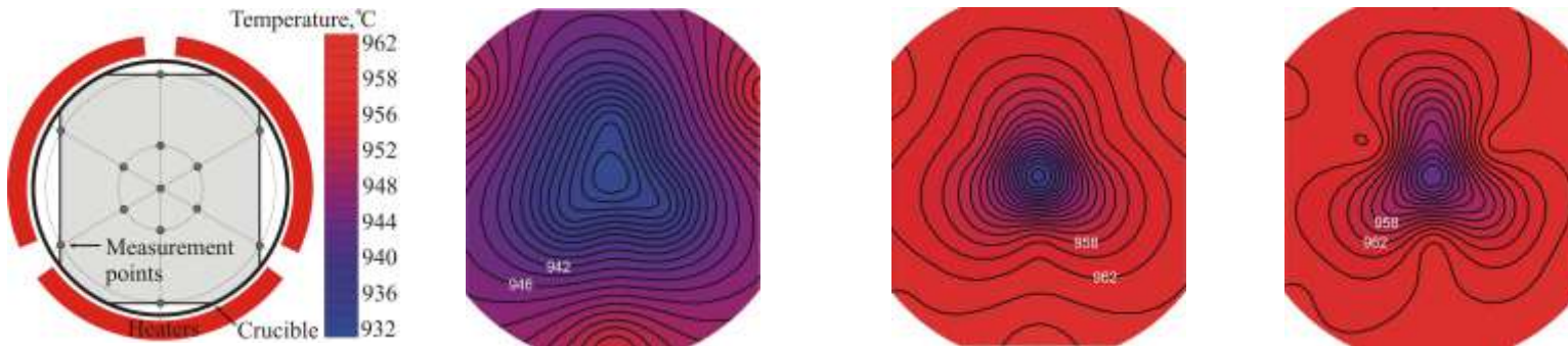
Fig. 3. (a) – measurement points and orientation of temperature distribution plots versus crucible and the heaters; (b, c, d) – temperature distribution in the horizontal plane at the level of melt surface, 5 mm and 20 mm below, correspondingly
