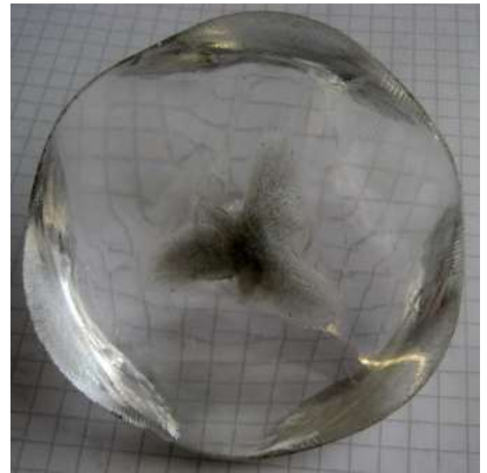
BBO crystal grown from BBO- \text{NaBaBO}_3 system, ___g. New design of the heater was used.
